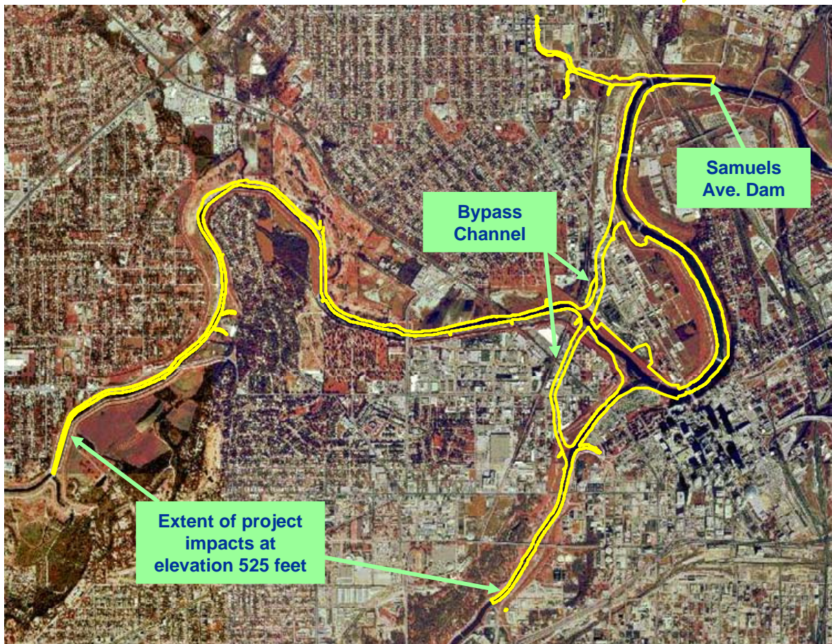
Figure 1 - Project area, features, and extent of water surface impacted by proposed project.
